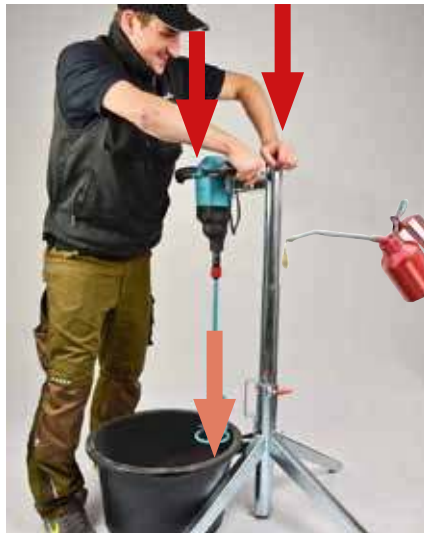
For mixing: push the machine into the material and move to all sides. To support while starting, press the tube with your second hand downwards to get the mixer lowered easily; grease the tube slightly
