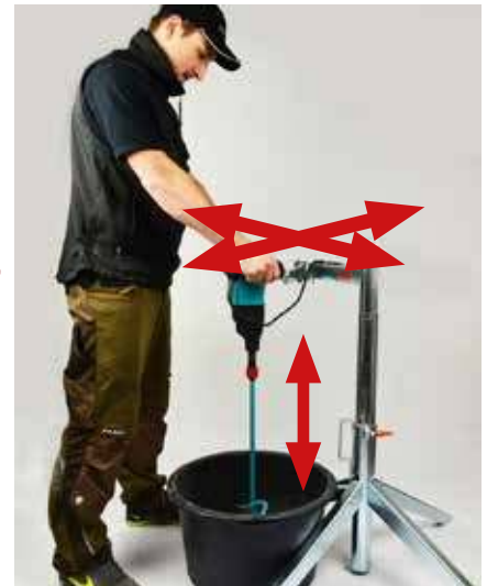
The machine cannot be operated on its own with the RMX. Always operate the mixing machine with two hands on the machine. Start up and run down the machine in the mixing container only. Ensure that the mixing container is stood in a firm and secure position. It is not allowed to block the ON-/OFF switch of the mixer for operation!
