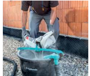
Placing the material bag on the teeth of the SHARKY creates a clean opening, whether paper or plastic bag.
